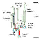
Figure – The replica of a water pressured reactor, with the hot and cold leg.
