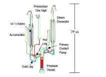
Figure – The replica of a water pressured reactor, with the hot and cold leg.
