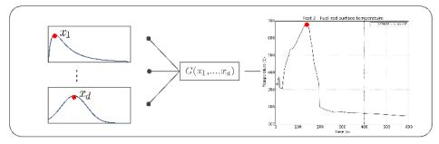
Our use-case is a thermal-hydraulic computer experiment (CATHARE), which simulates a intermediate break loss of coolant accident. The variable of interest is the peak cladding temperature.
